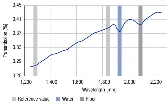
Fig. 2: NIR (transmission) spectrum with the measuring wavelengths used in TecoSens.
