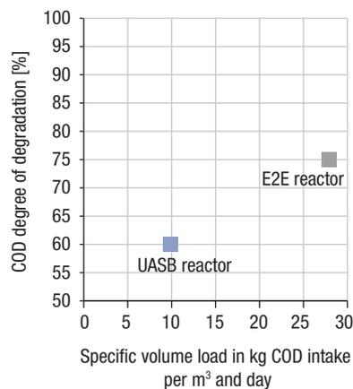
Fig. 2: Comparison of a UASB reactor with Voith E2E reactor.
