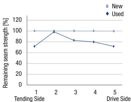
*Fig. 1: After being used by a customer for 446 days, the SynStron dryer fabric still had 72% of its original seam strength.*
