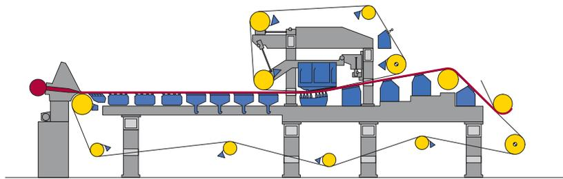
Fig. 3: DuoFormer D II for wood-free paper with extended speed range.
