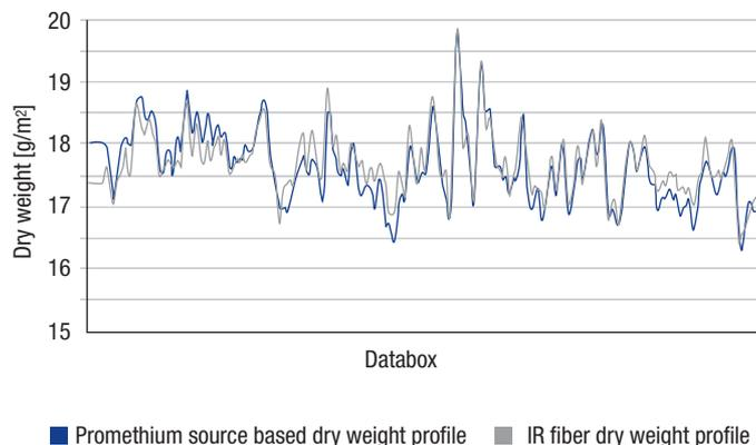
Fig. 3: Comparison of mean values (reel) derived from a conventional radiometric measurement and using Voith LSC TecoSens.
