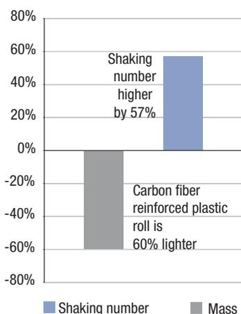
Fig. 3: Advantages of a carbon fiber reinforced plastic roll as compared to a steel roll.
