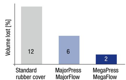
Fig. 6: Comparing the abrasion behavior of various rubber qualities.
