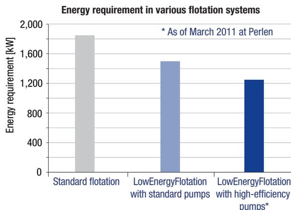
Fig. 3: Reduced energy requirement for flotation with the new LEF.
