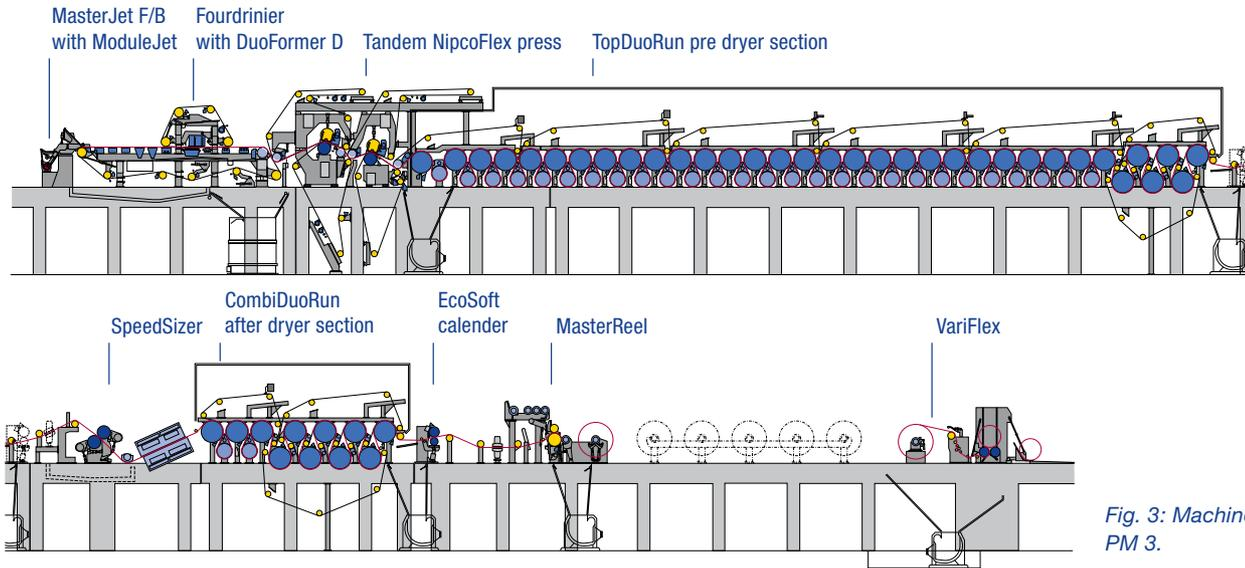
Fig. 3: Machine concept PM 3.
