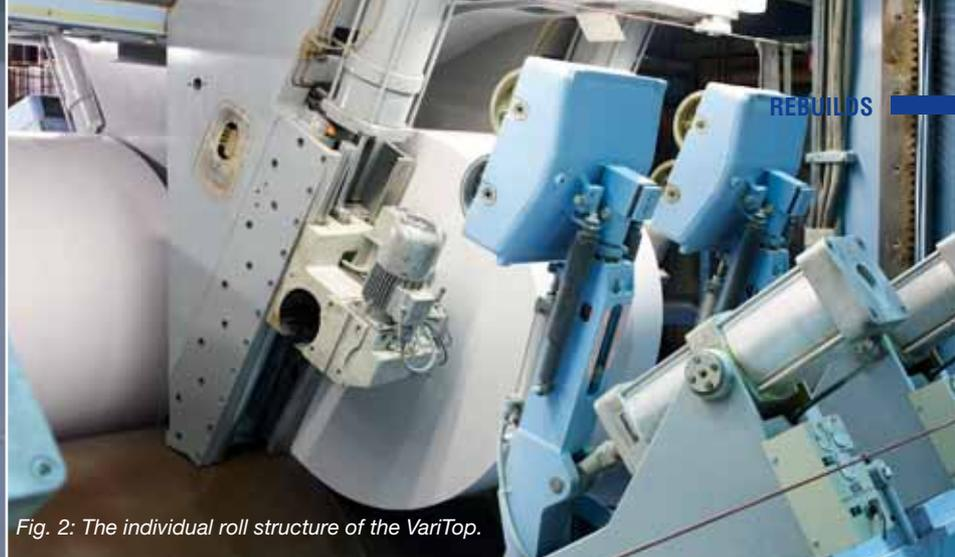
Fig. 2: The individual roll structure of the VariTop.
