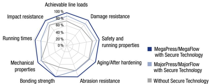
Fig. 5: Comparing the characteristics of the new Mega covers to Major and standard rubber covers shows impressively that the development goal of extending the service life was achieved.
