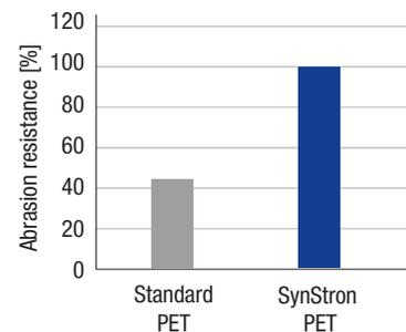
*Fig. 3: In comparison to standard PET, SynStron achieved, on average, 56% higher abrasion resistance.*
