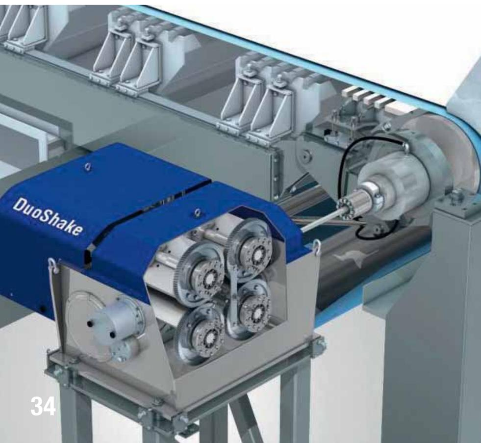
The CarboForm and DuoShake combination is already used in over 30 installations worldwide and is very successful in each one of them. A paper manufacturer in North America that produces testliner on a 4.7-meter-wide, two-layer Fourdrinier machine installed two DuoShakes together with CarboForm breast rolls in 2008 and 2009. The result was a clear reduction of the basis weight with identical strength values and increased machine speed.
