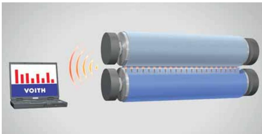
Fig. 3: A schematic diagram of the NipVision sensors.
