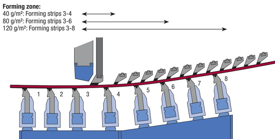
increase. Drainage boxes are fitted, tailored to the paper grades produced. Furthermore, instead of a suction couch roll, a high vacuum suction box is used as the last dewatering element. The first full scale installation confirms that this results in considerably lower investment costs and also reduced energy consumption.
