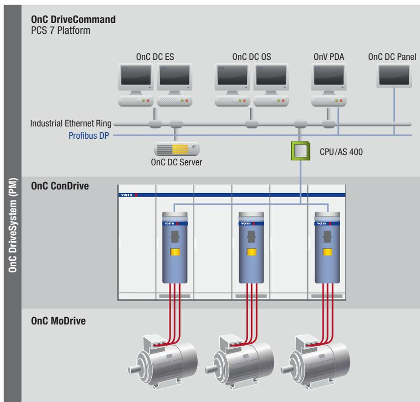
Fig. 2: The OnC DriveSystem comprises OnC DriveCommand, OnC ConDrive and OnC MoDrive. OnC DriveCommand integrates the drive control into the machine control system, allowing faster and more reliable optimization and troubleshooting.
