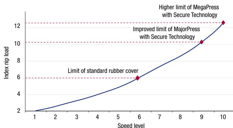
Fig. 1: The roll covers equipped with Secure Technology withstand noticeably higher nip loads than comparable rubber roll covers.
