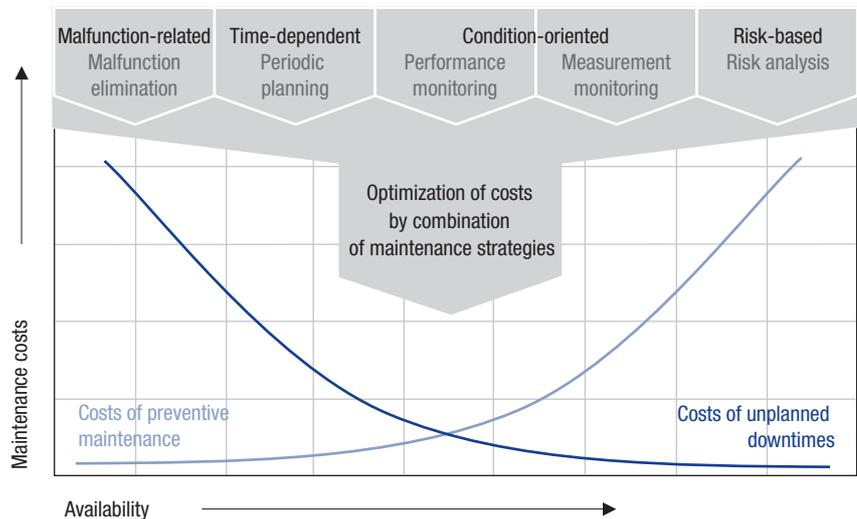
Fig. 2: Maintenance can be performed through various strategies. The right combination lowers costs for the paper manufacturer.
