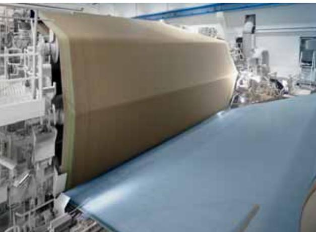
Fig. 1: Wire section and pick-up felt.
