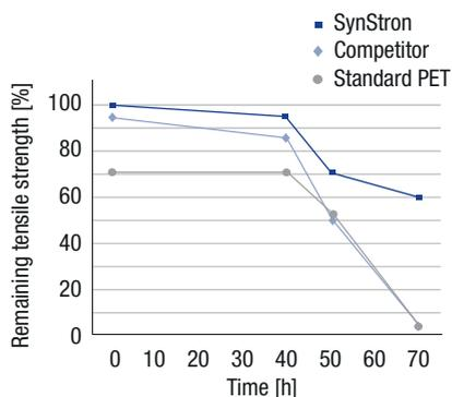
Fig. 5: While standard PET filaments have already torn, after 63 hours in a laboratory test, SynStron still has 60% of its original tear strength.
