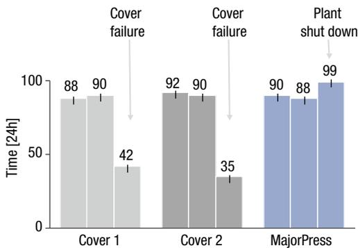
Fig. 4: The new rubber roll covers Major and Mega achieve longer running times in operation without problems.
