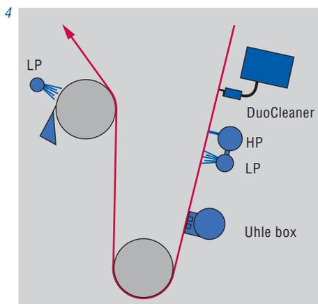
moisture profiling and increasing dryness can be located. The boxes are swiveled away during web threading.
