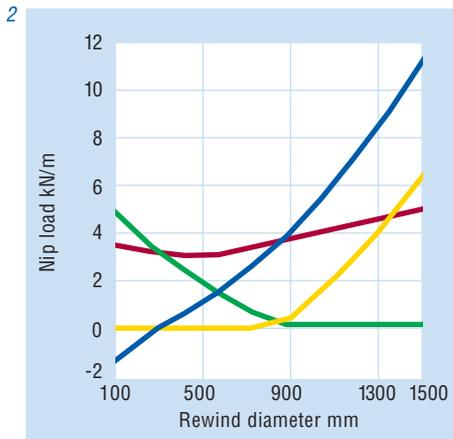
Fig. 3: Nip loads at two drum winder with soft covered drum #2.
