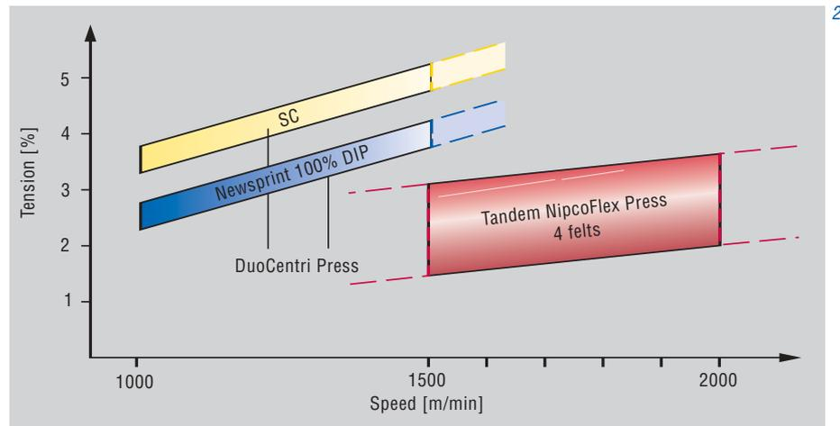
press sections need approx. 1.5% higher draw, Fig. 2. As further advantages of the closed draw configuration we expect less paper breaks, fast paper threading, no doctoring at center roll and high speed potential.
