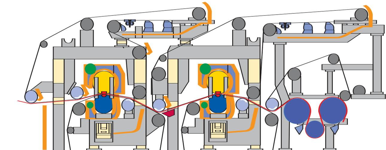
Fig. 4: Felt conditioning.
