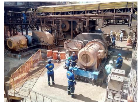
During test of the Voith start-up components
