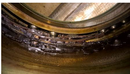
Destroyed bearing of the coupling in IND
