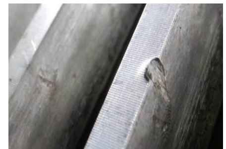
Detected damaged gearbox teeth
