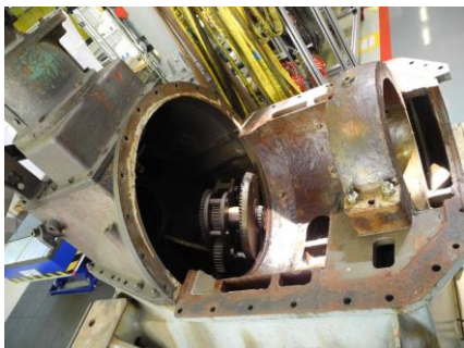
Condition of the planetary gear after delivery to Voith
