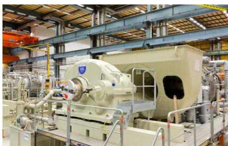
Caption: The turbo gear unit together with the gas turbine at Siemens, Sweden. (© Picture: Siemens Finspång)
