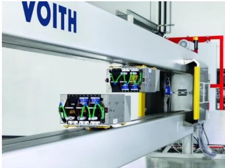
The new sensor generation features a compact, lightweight design and increases the reliability and availability of the machine direction controls.
