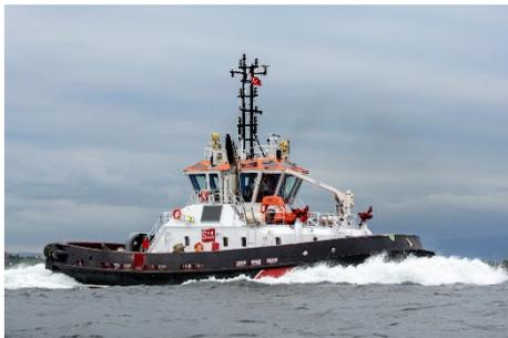
VectRA series tugs are high-performance VSP tugs in tractor configuration (Voith Water Tractors), designed for maximum efficiency.
