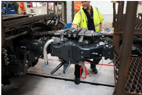
The successful installation of the four couplers at Green Cargo in Eskilstuna, Sweden, was carried out September 8-10, 2020.
