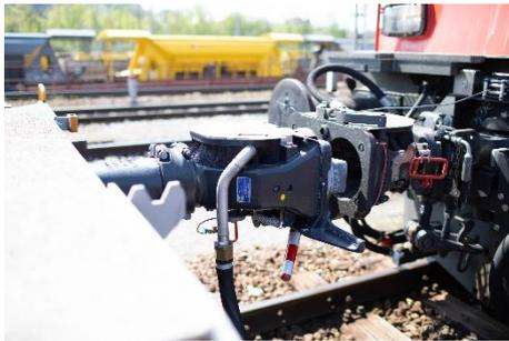
25 locomotives and 100 rail-cars from SBB Cargo have been equipped with Voith CargoFlex (Type 10) since May 2019.
