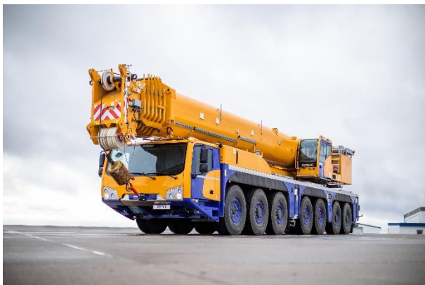
The AC 450-7 is equipped with a Mercedes-Benz driveline with a wear-free Turbo Retarder Clutch from Voith.
