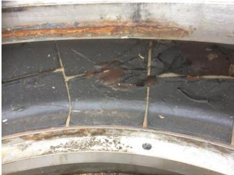
The basalt inner lining of CombiSorters had to be replaced every year. To counteract this, Voith has now developed a special cast steel.
