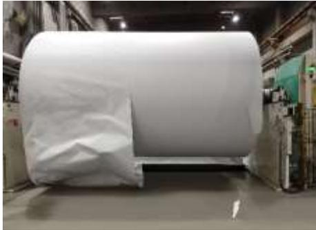
With the help of the TailFix, paper ends can be reliably fixed. The picture shows the condition without outer layer gluing on the left and the optimized condition after using the TailFix automatic gluing system on the right.
