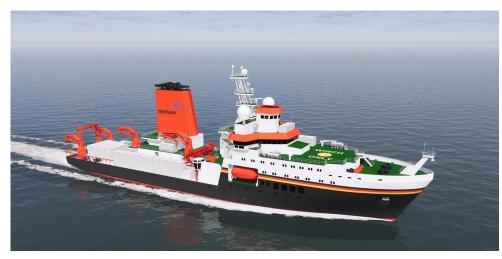
Research vessel Meteor IV of the Federal Republic of Germany with two electric Voith Schneider Propellers (eVSP) and a Voith Inline Thruster (VIT). Image source: FR. FASSMER GmbH & Co. KG
