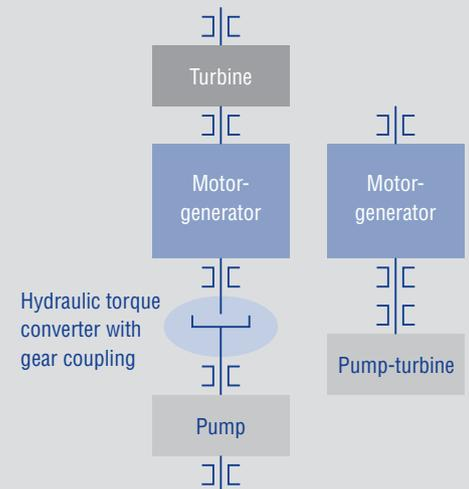
Comparison of a separate pump storage arrangement (left) and a reversible pump-turbine (right).
