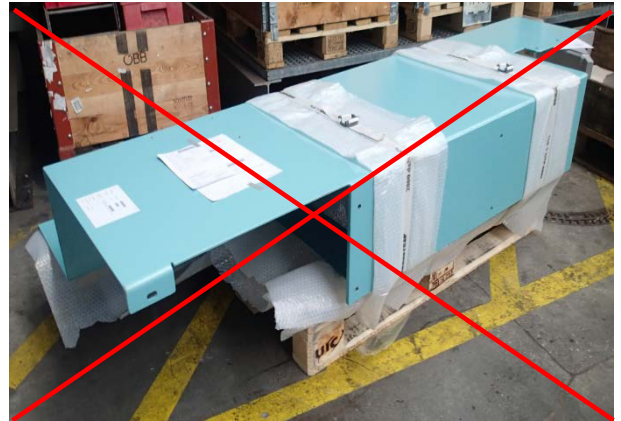
Figure: Incorrect pallet packing
