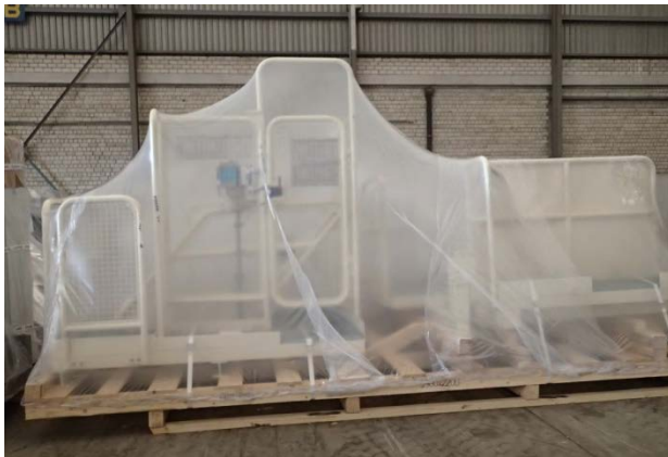
Figure: Correct pallet packing
