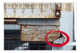
→ The wire mesh is so torn that the wire ends extend to the inside or outside, (one missing mesh per side is allowed),
