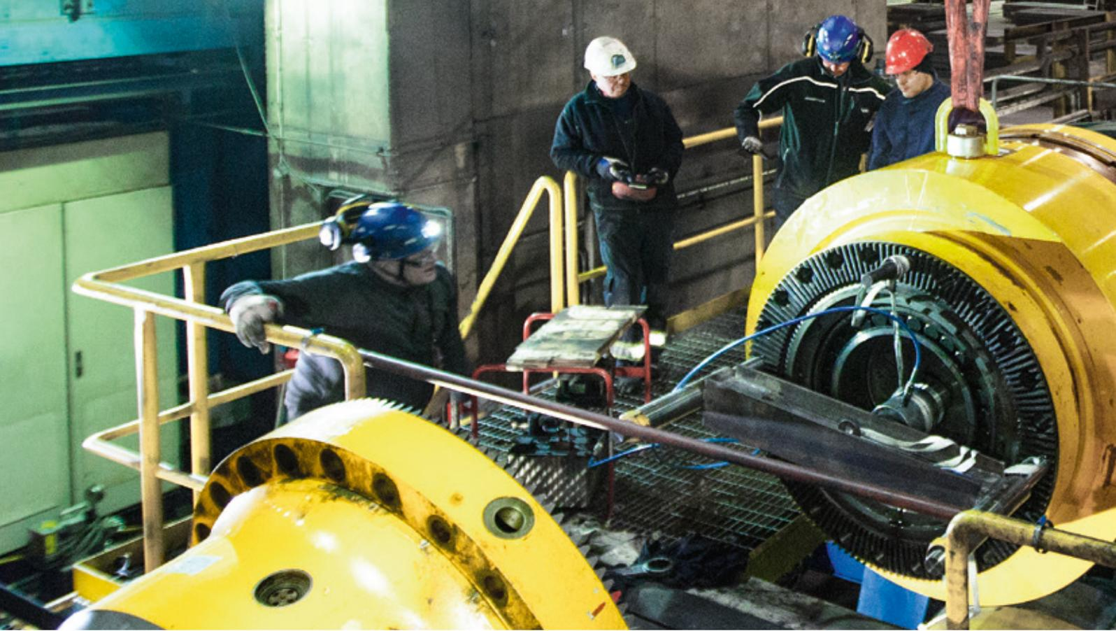
**SSAB utilizes Voith torque limiting couplings to protect valuable equipment at its heavy plate mill in Oxelösund, Sweden. The Voith couplings protect the drivelines from overloads during production and therefore help ensure that the equipment works reliably and efficiently at a maximum level.**
