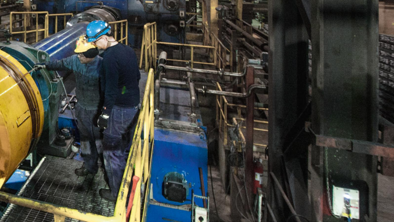
At Voith's site in Hudiksvall, 400 kilometers north of Oxelösund, worn couplings are repaired and made fit for reuse. Two SafeSet torque limiting couplings are currently in use in Oxelösund. To ensure downtimes are as short as possible in the event of overload, SSAB keeps one spare SafeSet coupling in stock.
