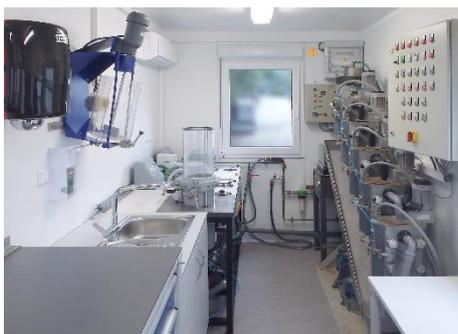
The Voith MobiLab is a fully equipped wet laboratory for analyzing stock samples directly on site.
