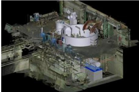
With the 3D Scan, Voith experts on site can create a digital spatial image of a machine and its environment.
