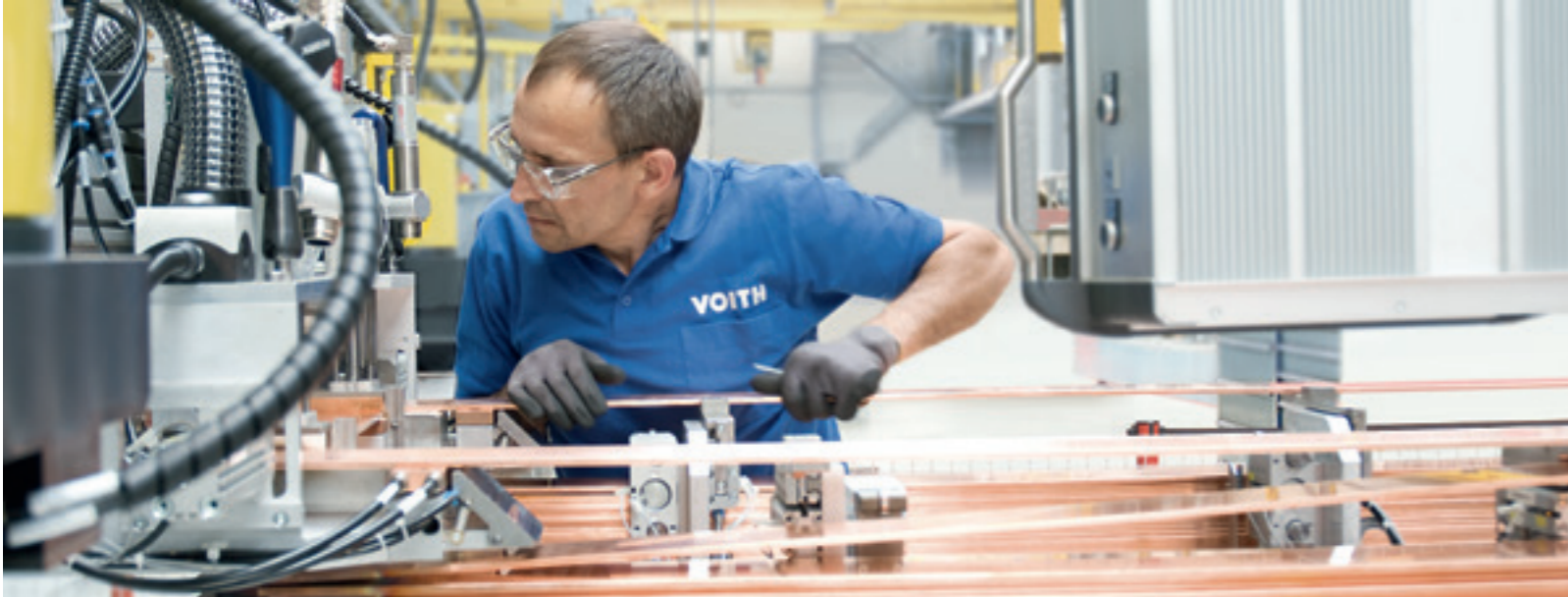
Pole coil brazing and lamination
