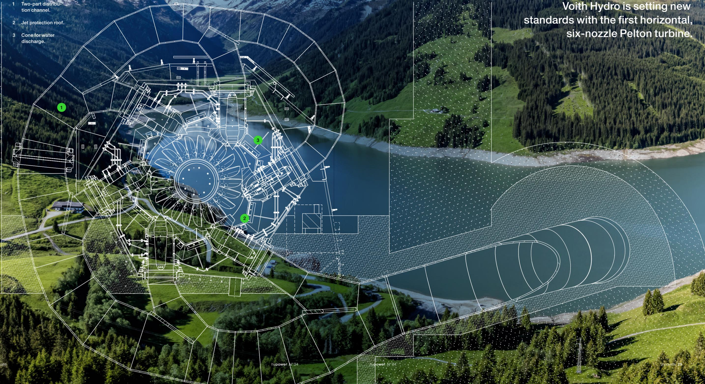
One particular challenge has kept Voith Hydro's development engineers busy for more than 10 years: What if we could arrange Pelton turbines with three or more nozzles horizontally without sacrificing performance, instead of vertically, as is the norm today?
