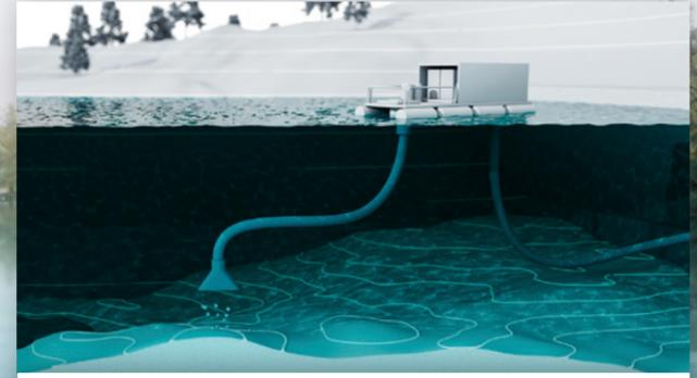
At the heart of Voith's SedimentCareProgram is a fully automatic boat. Sediments are sucked from the bottom through a pipe and transported in low concentrations via a pipeline to the hydropower plant.
