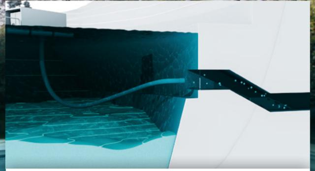
The stirred-up sediment particles pass through the pipe into the penstock and can simply pass through the turbine with the flow of the water.
