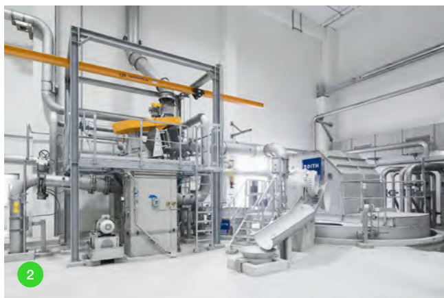
2 The Twin Pulp System with IP-R Pulper and IntensaMaXX at Schoellershammer in Germany.
