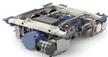
Caption 1: The RailPack DE uses an electric generator for power transmission.
