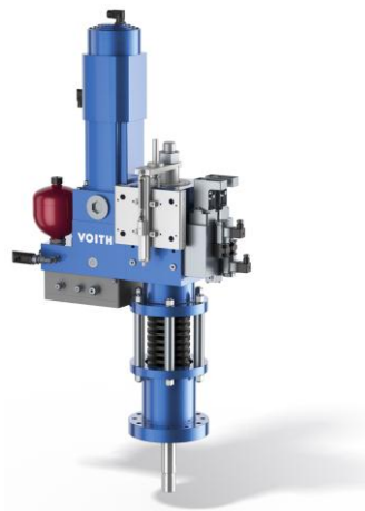
Figure 1: The Voith self-contained linear drive with fail-safe function. It regulates control valves on turbines precisely and in a highly dynamic way.
