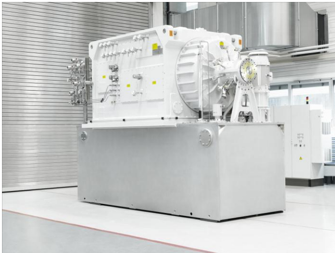
Fig. 1: Voith's variable speed planetary gearbox 'Vorecon' controls the speed of compressors on the FPSOs in the 'Pre-Salt Cluster' off the coast of Brazil.
