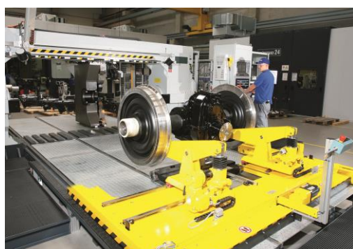
With the wheelset press in Heidenheim Voith assembles wheelsets
