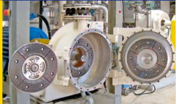
TwinFlo refiner with energy-saving Pluralis filling.
