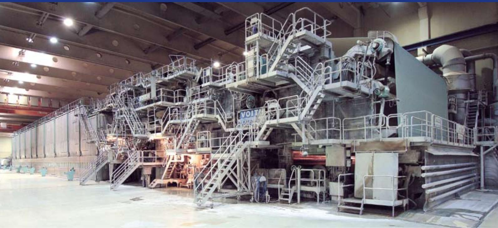
The PM 4 at UPM Steyermühl was rebuilt to the modern DuoFormer CVB design.
