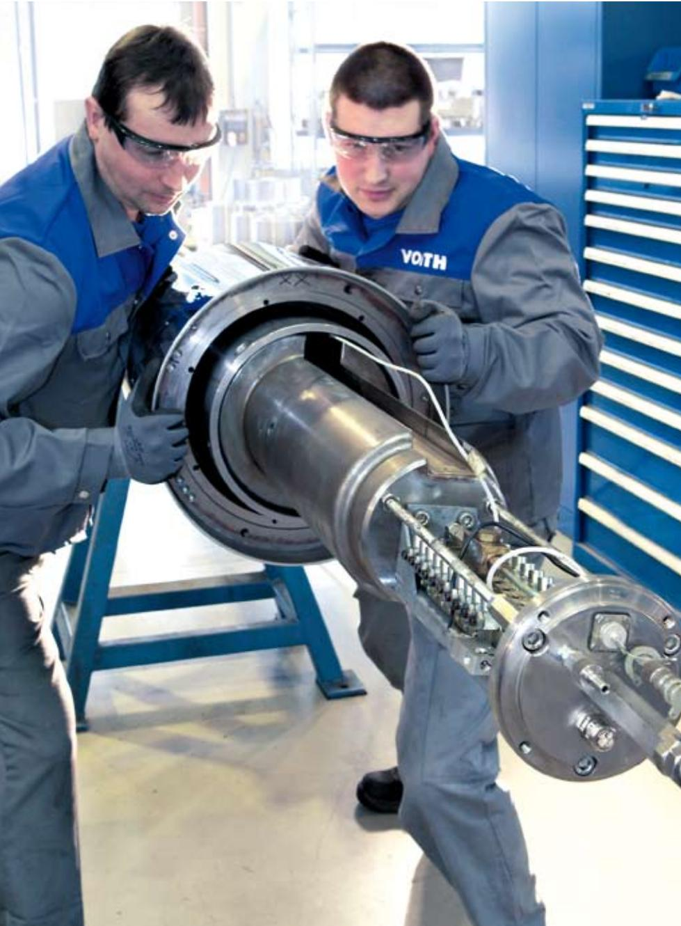
*Disassembling of a spreader roll.*
