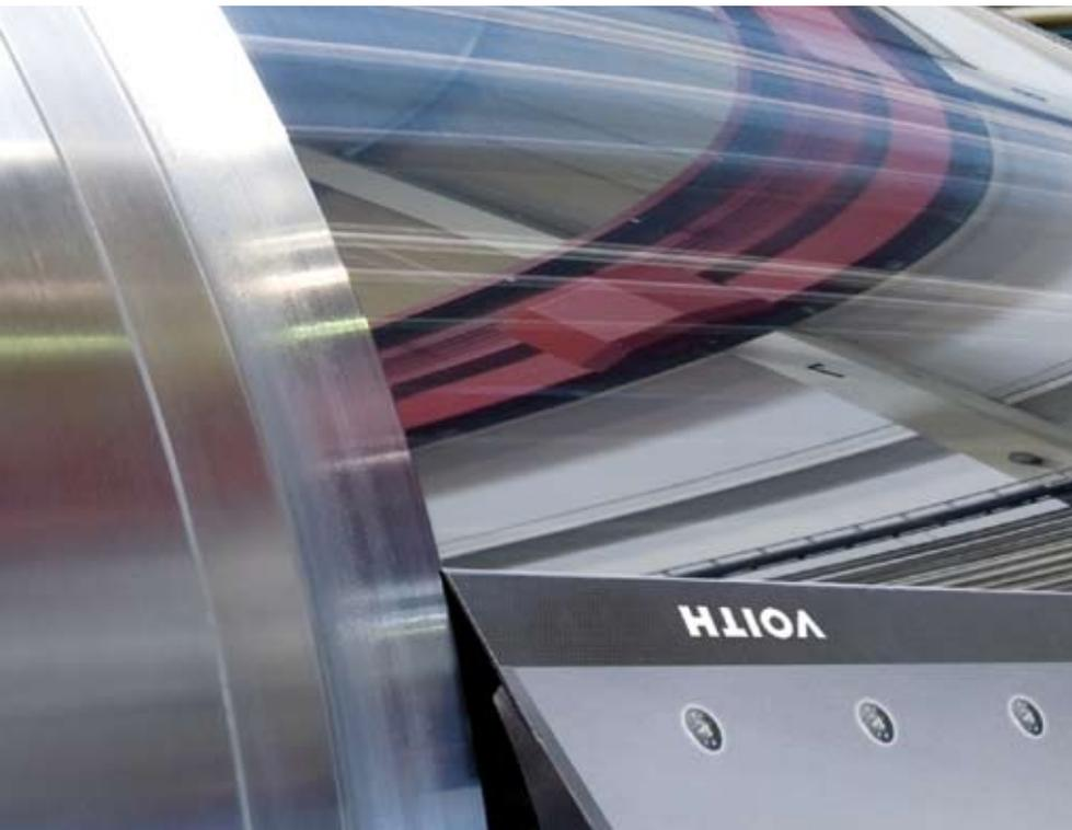
At Norske Skog Bruck in Austria, doctoring deposits in the third press were affecting the operating properties of the central press roll. The use of >>> SkyTop doctor blades over a longer period reduced doctoring deposits and extended blade life from 14 to 21 days.
