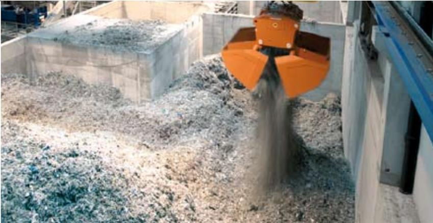
*An intelligent self-propelled crane system takes fuel out of storage and feeds the secondary treatment stages, mixing and feeding systems.*
