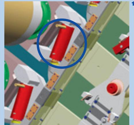
**Fig. 1:** Compensation cylinder.
