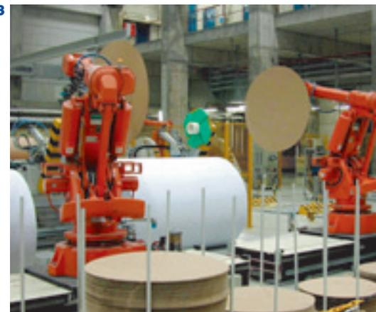
**Fig. 1:** Twister™ wrapping and folding station.
