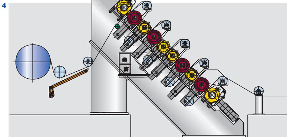
hand the CD thickness profile is optimized, which significantly improves runnability in the coating machine, and on the other hand moderate precalendering makes for more efficient calendering.
