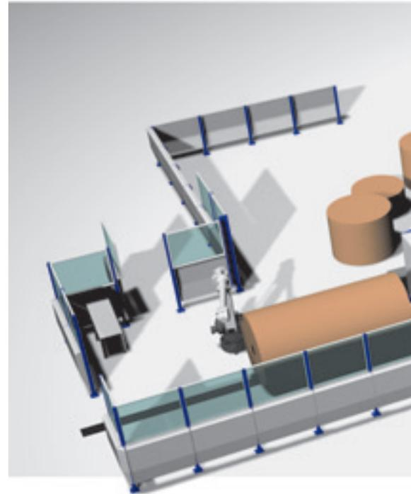
The double claw of the outer header robot automatically adapts to various diameters. Here again, the headers are taken directly from the pallet stack, a special separating device ensuring that even if firmly linked together, they are removed individually. As soon as the header press tilts into position, the robot places the outer headers precisely on the pressure plates, which can be as hot as 180° C.
