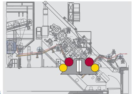
itoring and roll edge cooling by the Soft-rol™ system, threading with open nip, etc.
