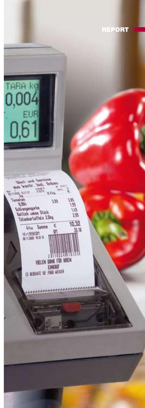
Checkout receipts are printed on thermo paper.
