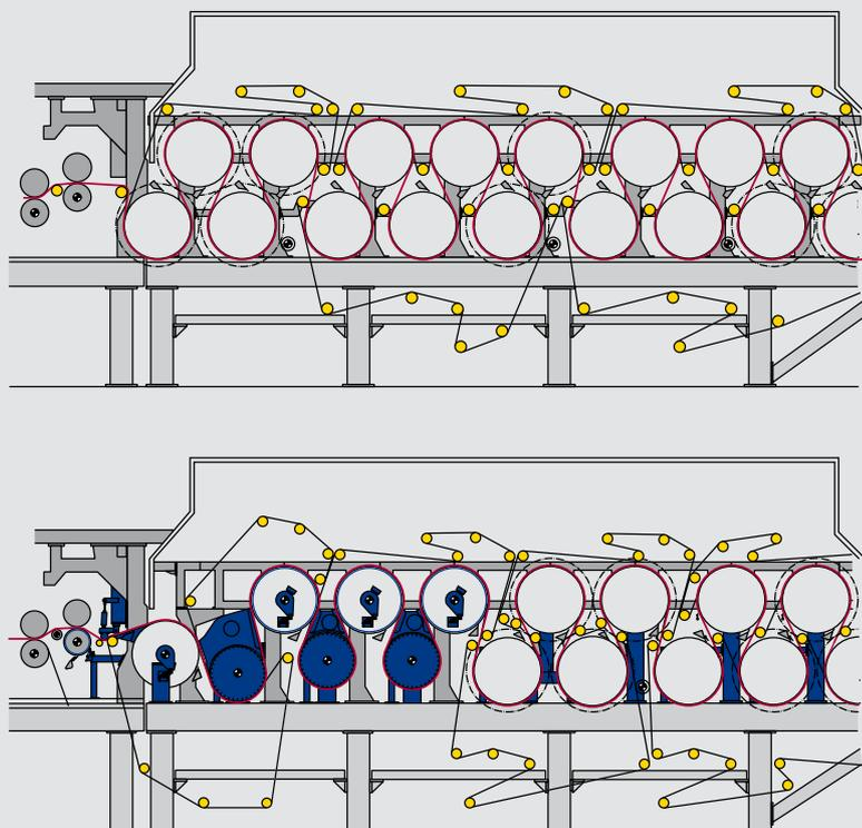
*Before the rebuild by Voith Paper, the paper machine in Besozzo was a fourdrinier machine with dandy roll producing décor paper. The rebuild now makes it possible for the PM 4 to produce masking tape as well.*
