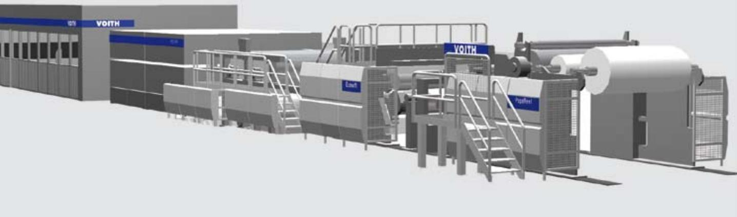
embedded into the paper. Both of these authenticity attributes are worked into the paper during the forming section of the machine. The double-layer forming system from Voith Paper, which consists of the Master-Vat and the ShortFormer B, makes Voith the market leader in this technique. Nearly all European banknote paper mills produce the second paper layer using the ShortFormer B that Voith Paper has continued to develop.
